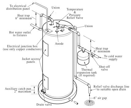
A new combination temperature and pressure relief valve, complying with the Standard for Relief Valves for Hot Water Supply Systems, ANSI Z21.22, is supplied and must be installed in the opening provided and marked for the purpose on the water heater. No valve of any type should be installed between the relief valve and the tank. Local codes shall govern the installation of relief valves.
